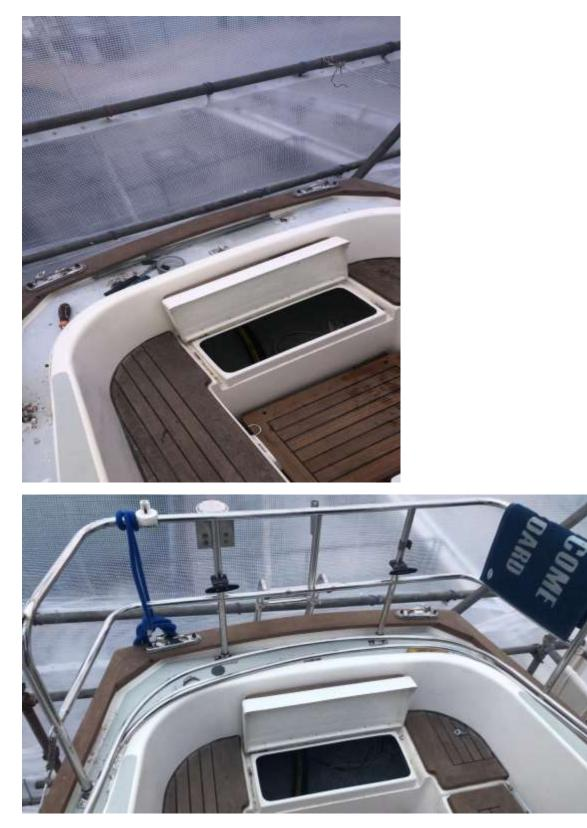
In the photos above I had to dismantle the stanchion posts so that the deck could be sanded and primed so that a new cork deck could be fitted. The
