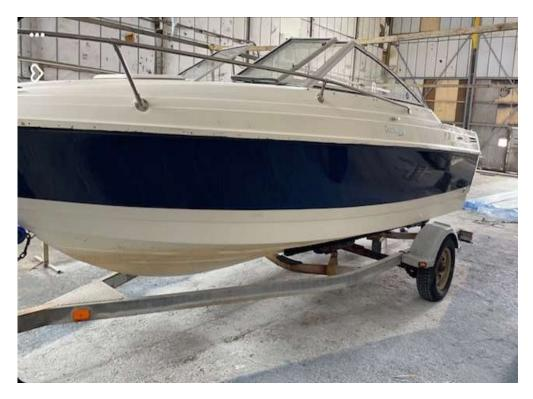
We are also in the process of professionally applying copper coat antifouling on the hull which is almost compete.
