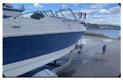
After that I applied a base coat of epoxy which acted as a great guide for the next step which was a fair and fill. Epoxy highlights any dips and scratches that would cause the respray to not look the correct standard that my employer would expect. Epoxy is also great for added protection on the hull.
