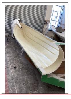
At college recently I have been studying fibreglass repairs in grp hulls, this involves making a 30mm hole in the hull of a dinghy below the waterline. We then seal the hole with tape and rebuild the structure from the outside in, starting with layers of gel coat and then progressing onto layers of grp. The knowledge I have learnt from this will also help me in other types of repairs I might undergo at work, such as repairing air blisters in a piece of fibreglass.
