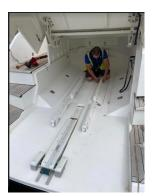
This image is of me removing a simple tender launch system as the customer requested an easier, more efficient launch system was installed. The main structure was removed and the glue residue was cleaned.
