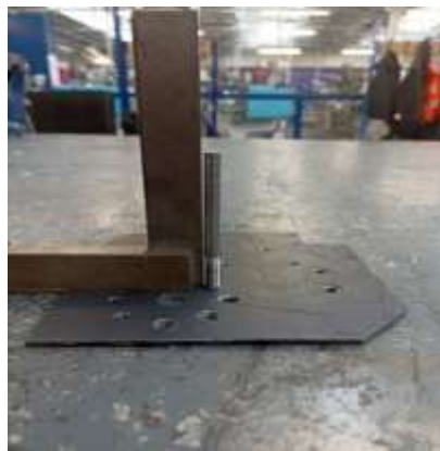
A practice plate complete with threaded M6 rod made at college.
