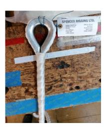
Spencer Rigging carried out a re-rig of a classic gaff rigged yacht which is now based in the south of France. We completed a new set of standing and running rigging. I was involved in the rope work. This involed some traditional finishing, including leathering to the splices and three examples of this are shown in the photos below.
