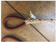
For one of our industrial customers I have been involved in a project to seize some cable. This is similar to the whippings I have done with rope, but more complex and intricate as it is done with a special seizing wire. The picture below shows the finished seizing.
