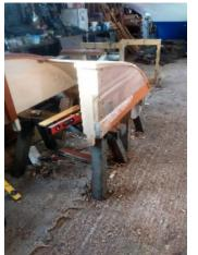
rotten it was replaced with a piece of oak shaped to fit the deck cut out, I used stainless steel screws to fix the new planks to it and used West epoxy glue to make a strong joint.
