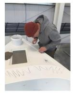
Here is an image of me using wet and dry sandpaper to perform a gel coat repair on the Duchy 21 deck.
