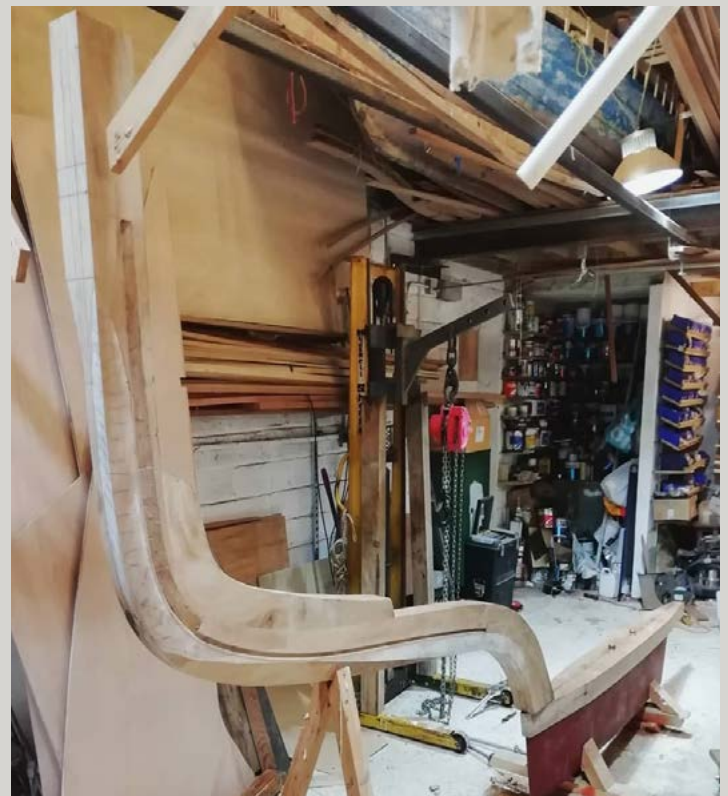
Cutting the rabbet on the stem and then glueing it in place.
