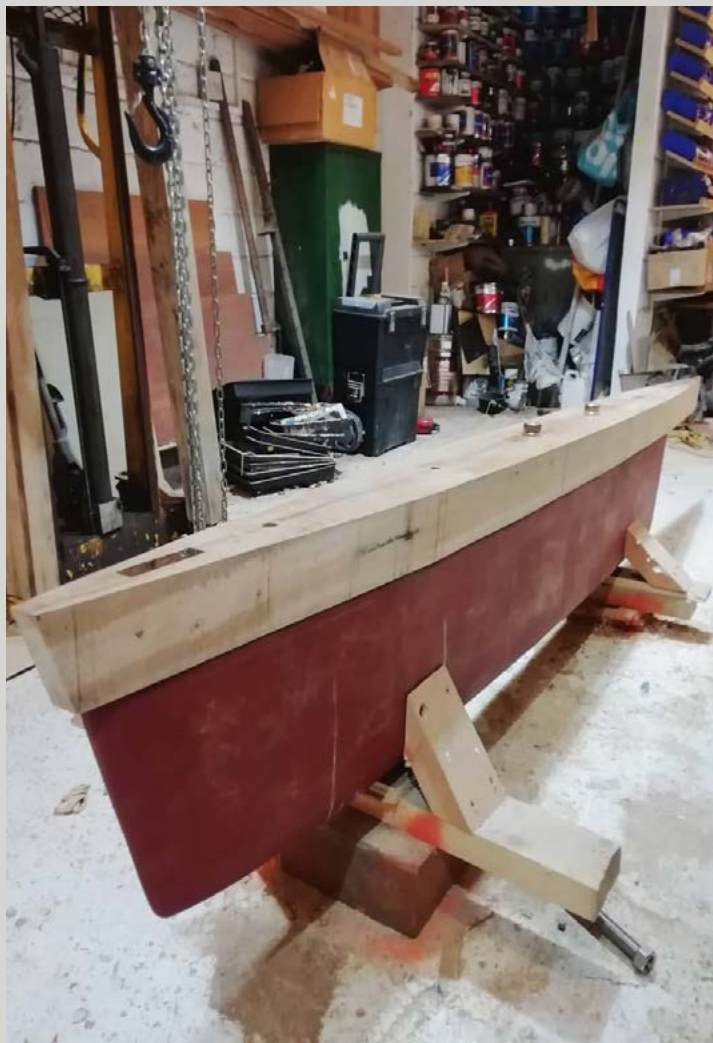
Setting the ballast keel and bedding the wooden keel on top - also shaping the stern post
